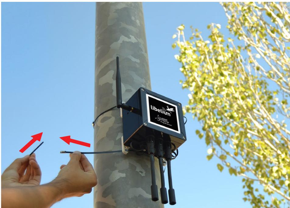
Figure : Placing Waspmote Plug & Sense! on a street light
