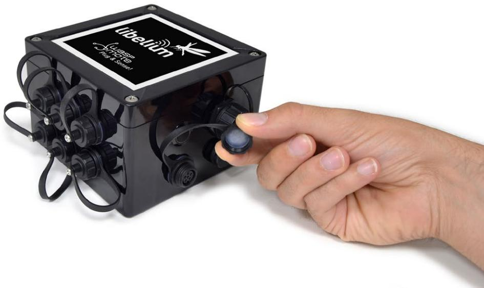
Figure : External solar panel connector
