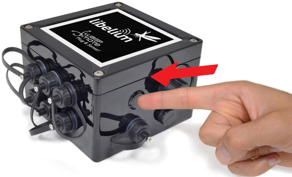
Figure : Turning on Wasp mote
