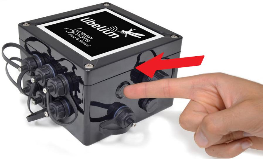
Figure : Turning on WaspMote
