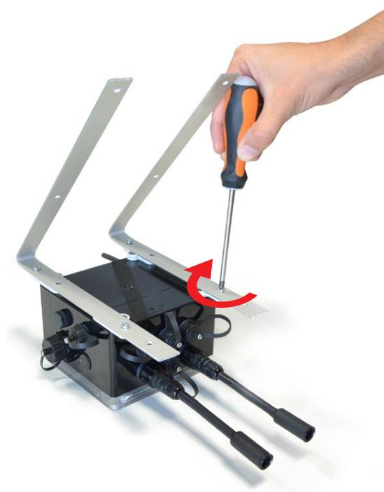
Figure : Securing the solar panel bracket to Wasp mote
