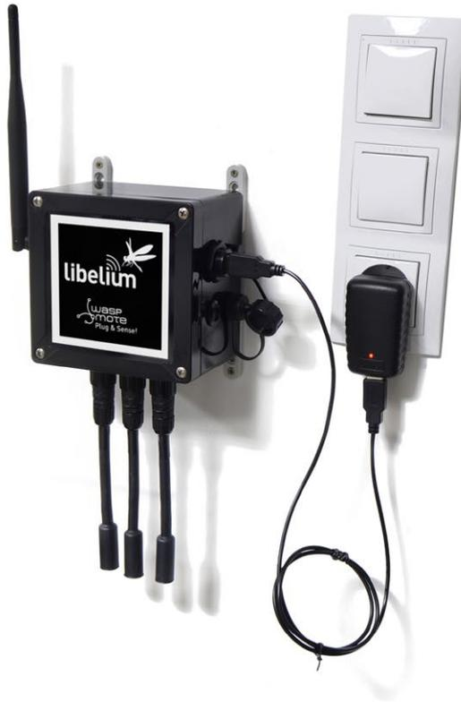
Figure : Charging the mote via USB
