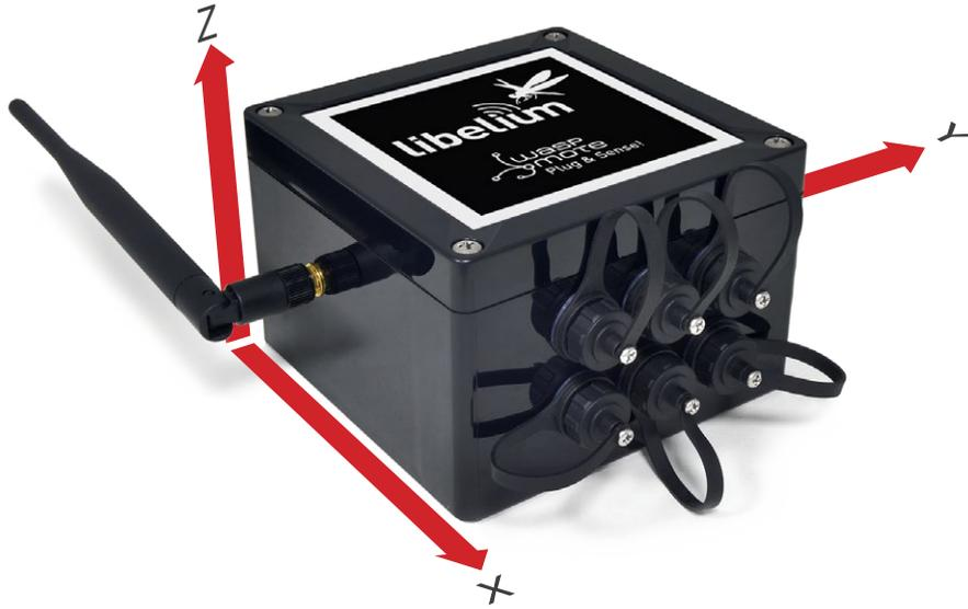
Figure : Axis direction in Waspote Plug & Sense!
