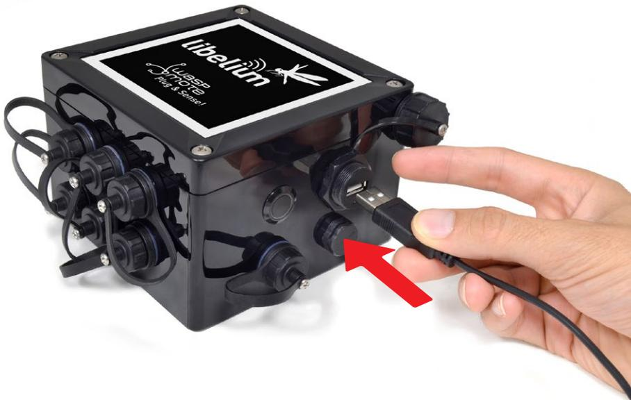
Figure : Connecting the USB cable to Wasp mote
