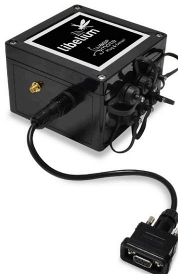
Figure : DB9 probe connected to Plug & Sense!
