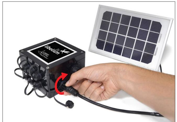
Figure : Connecting the solar panel to Wasp mote Plug & Sense!
