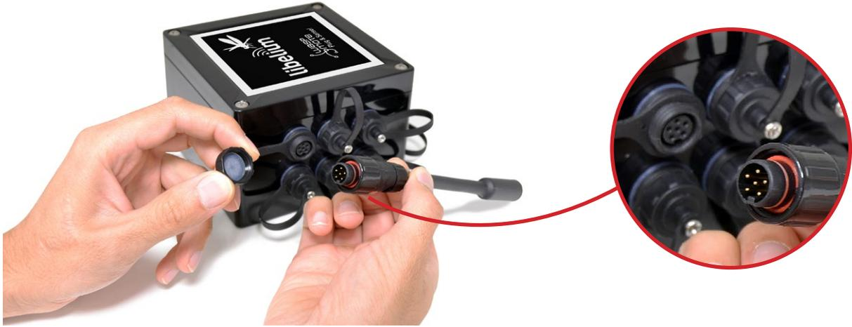
Figure : Detail of sensor waterproof connector
