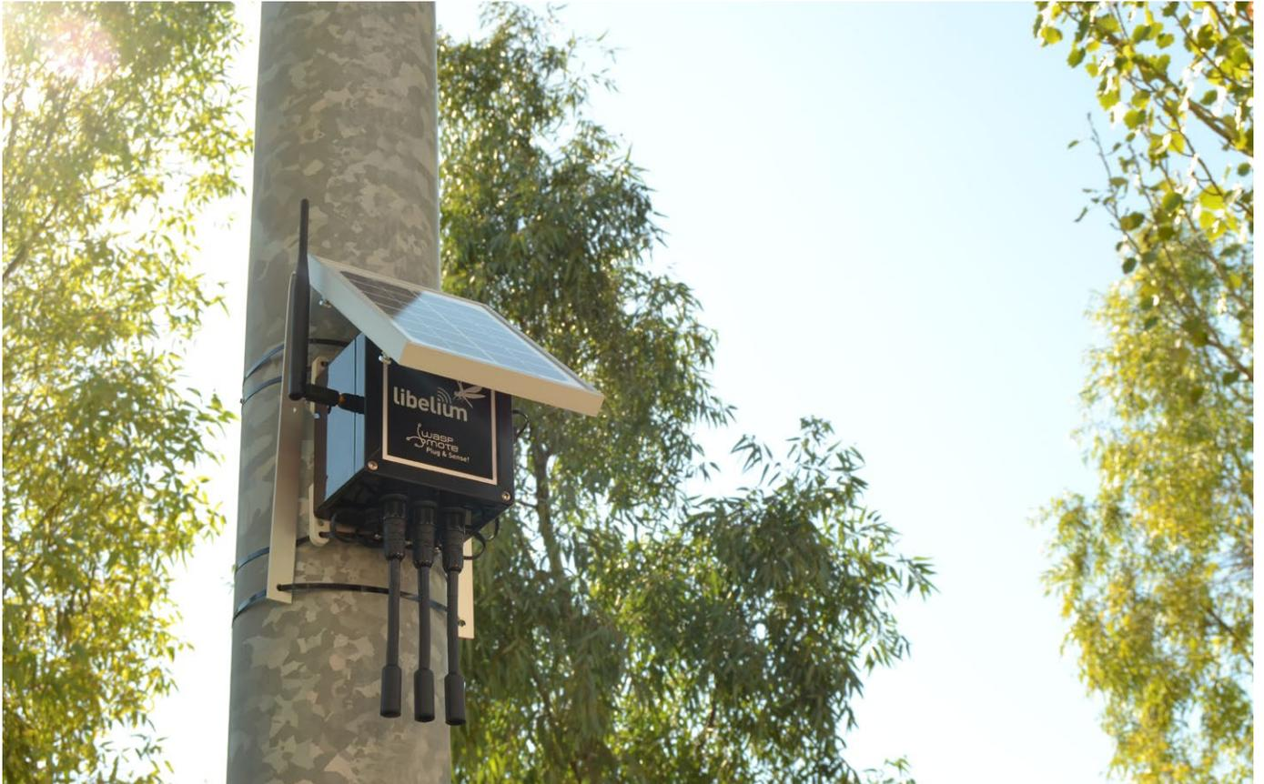
*Figure : Typical installation of the external solar panel*
