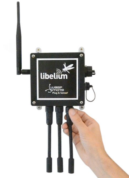
Figure : Connecting a sensor probe to Wasmote Plug & Sense!
