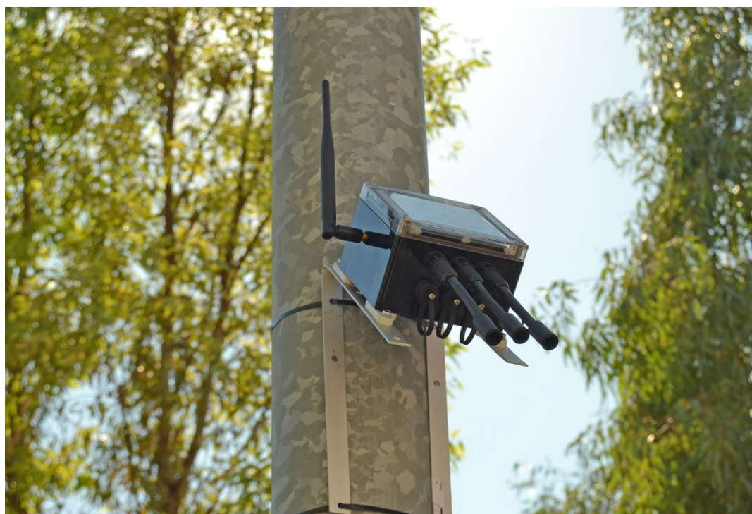
Figure : Wasmote Plug & Sense! powered by an internal solar panel
