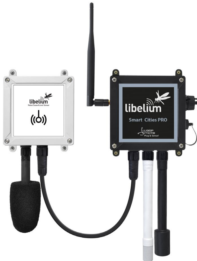
Figure : Connecting the data cable to the associated Plug & Sense! Smart Cities device
