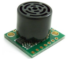
Figure : Ultrasonic I2CXL-MaxSonar®-MB1202 from MaxBotix™ Sensor
