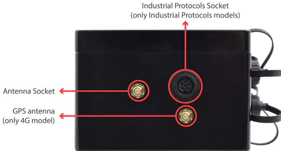
Figure : Antenna side of the enclosure
