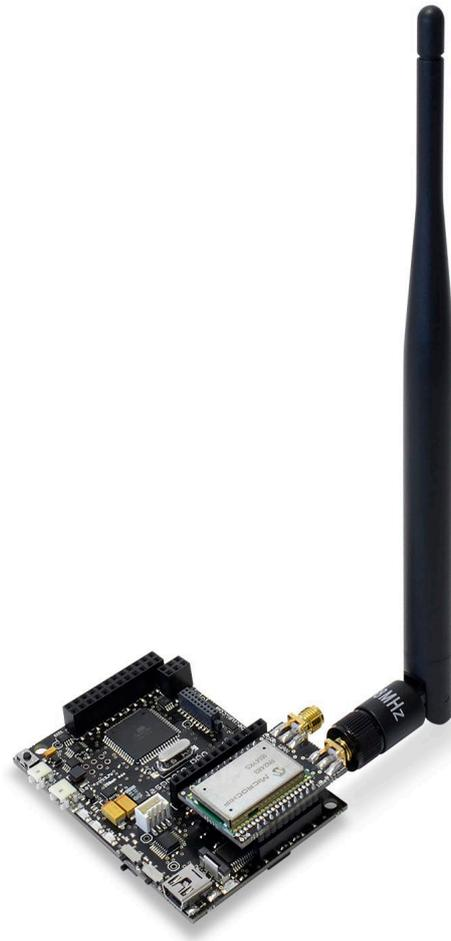
Figure: LoRaWAN module in `SOCKET0`
