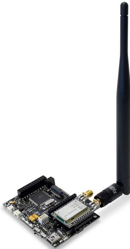
Figure: Waspote LoRaWAN
