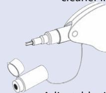
Flip-open cap for inserting connectors for cleaning
