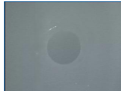
Improperly Keyed APC Connector
