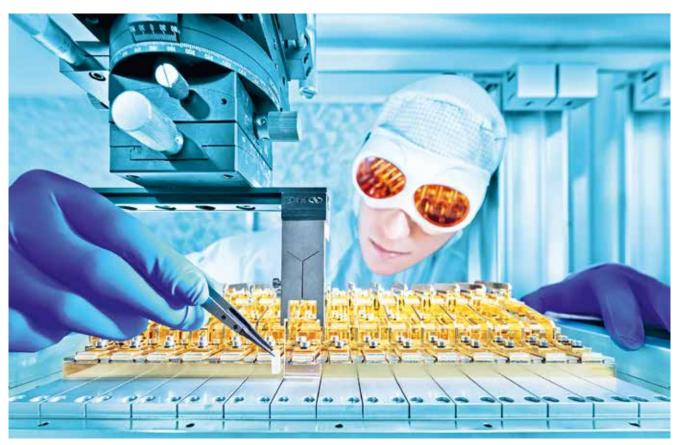
Because the laser line is separated into 15 individually controlled line segments with an area of 1.5 mm by 21 mm, the laser beam strikes only the specifically desired welding points on the plastic parts (figure: Limo/Markus-Steur.de)
