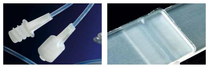
Fig. 5. Using vibration stimulation and absorbance, diode laser systems with a wavelength of 1,470 nm can even heat transparent, white and semi-transparent polymers (figures: Limo, Fraunhofer ILT for the EU-funded PolyBright project)
