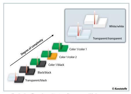
**Fig. 4.** The absorber effect makes combinations of transparent and black components easy to join with laser transmission welding, whereas the pair white/white is the most difficult (figure: Treffert)
