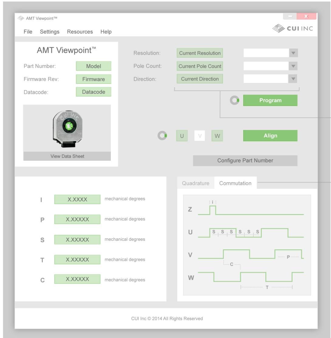
AMT Viewpoint has a waveform graph tool that allows the user to see what the timing is for each signal based on the resolution that is selected. These values are expressed as mechanical degrees and a simple calculation by the user can determine precise time values.
