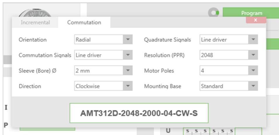
The AMT Viewpoint contains a tool that allows you to create AMT11 and AMT31 part numbers for direct ordering from CUI. To access this tool navigate to:
