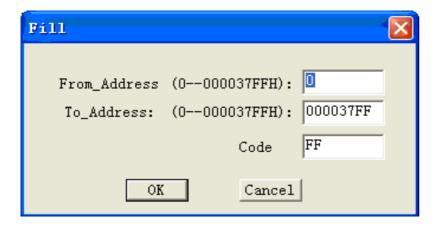
This selection will bring up the Fill buffer dialogue box. It consists of the Start address input line, End address input line, Fill data input line, OK and Cancel buttons. Input any desired data to be filled into the Fill data input line, and specify the range by indicating the beginning and ending addresses. For the Fuse buffer edit window, the data will be either 1 or 0. For the Data buffer edit window, it will be a two-character HEX code.
