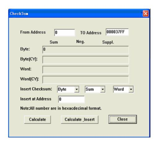
The checksum dialog is used for calculate checksums of selected block in buffer. The checksums are calculated by next way:
