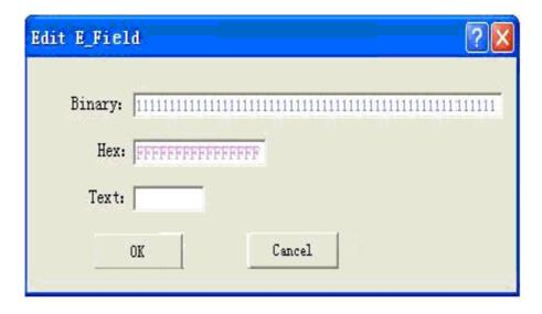
This option is only used for PLD. It used to edit information in the area. It also can be edited in the buffer. The size of E-Field is 64 bit. It includes site of seat, fig mode, version and so on.
