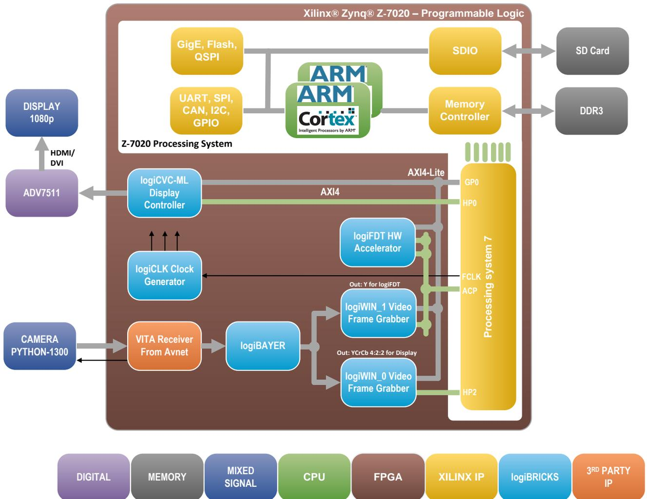
**Figure 25: logiREF-FACE-TRACK-EVK Reference SoC Block Diagram**
