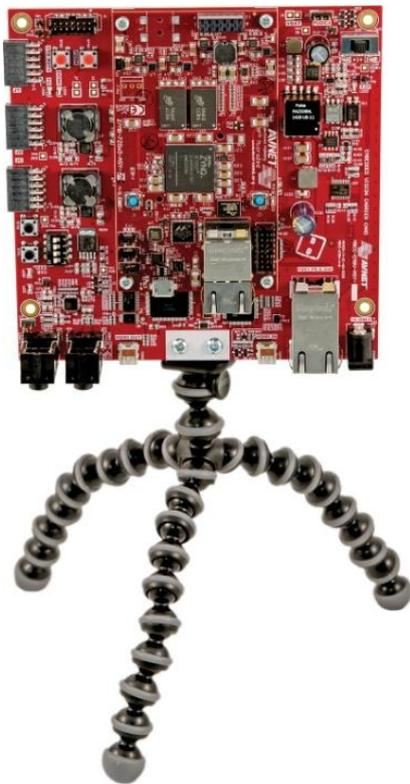
**Figure 2: Avnet MicroZed Embedded Vision Kit**
