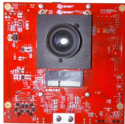
**Figure 31: The PYTHON-1300 Camera Module Plugged In the Carrier Card**
