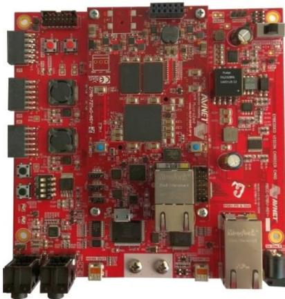
**Figure 30: The MicroZed Board Plugged In the Carrier Card**
