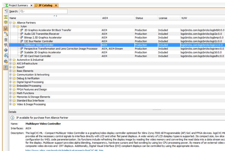
Figure 3: logicBRICKS IP Cores in the Vivado IP Catalog
