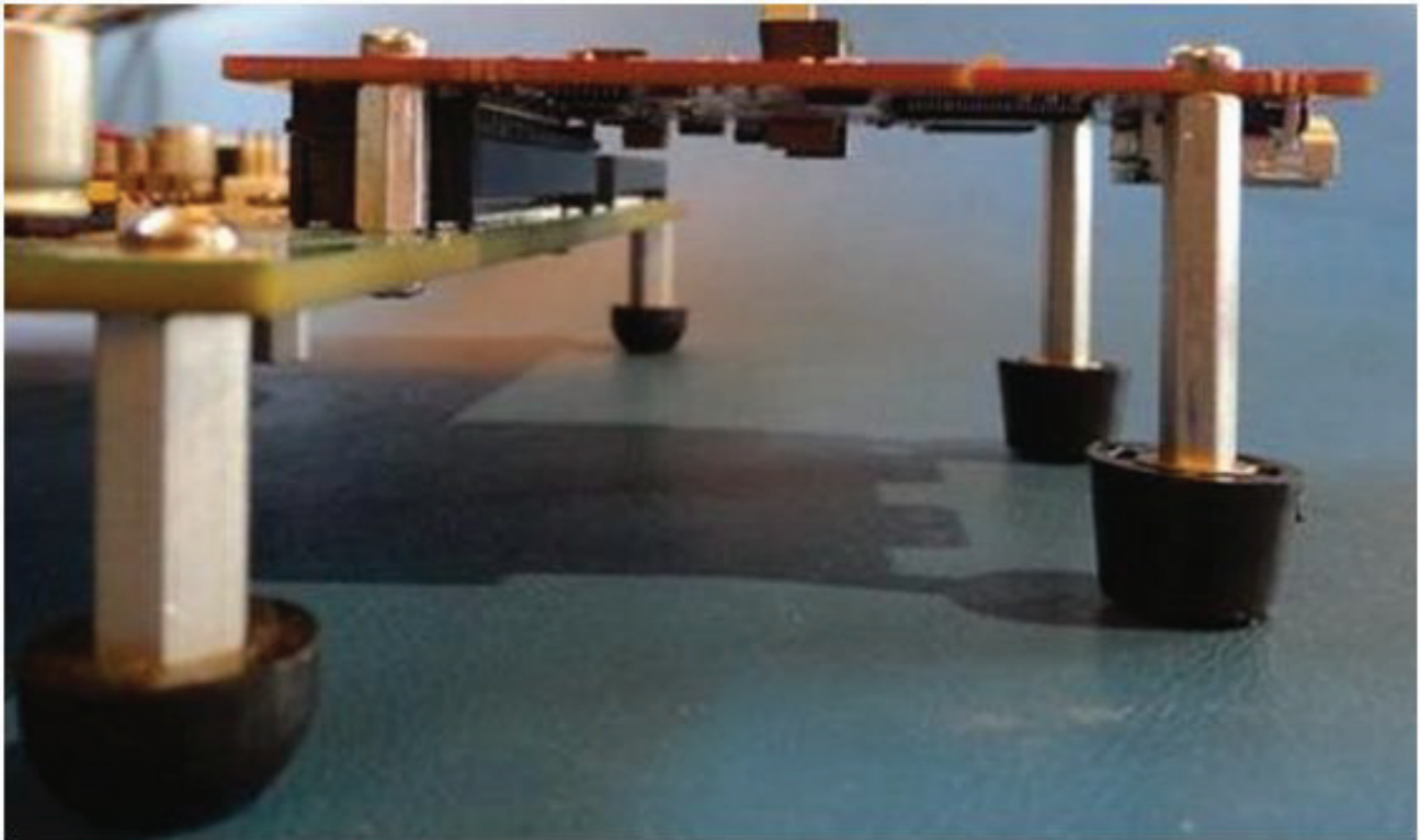
Figure 3-3: ZVIK FMC Mounting Hardware Detail
