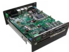
**Cable Free Design** All components and connectors are directly mounted on the PCB using SMT and DIP without any connecting cables. This eliminates possible cable failure and also prevents signal degradation and latency. Our cable free design results in an extremely strong and durable mechanical structure which is suitable for the harshest environments.
