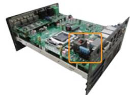
Exchangeable Fuse Socket
