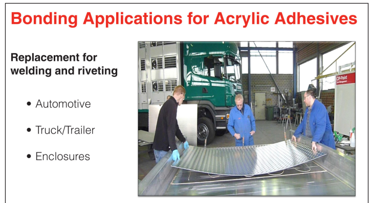
Figure 4: Next-Generation acrylic adhesives are an ideal replacement for welding and riveting joining methods in automotive, truck/trailer and enclosure applications.
