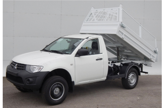
Figure 6: The new design for this utility truck bed required a change in the assembly method from welding to adhesives.
