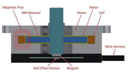
Torque feedback to the operator is generated through our proprietary "Direct Shear Mode" design in which a rotor attached to a shaft shears magnetically responsive (MR) material against a fixed stator. As the current commanded by the vehicle steering controller to the TFD steering unit changes, a low-power (0-1 amp) coil generates a magnetic field that instantaneously changes the properties of the MR material and the subsequent torque feedback.
