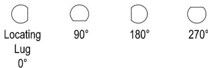
NOTE: The angle of the spindle flat is shown with the locating lug at the bottom of the switch, when the switch is set in the fully anticlockwise position (i.e. position 1) viewed from the knob end of the spindle.
