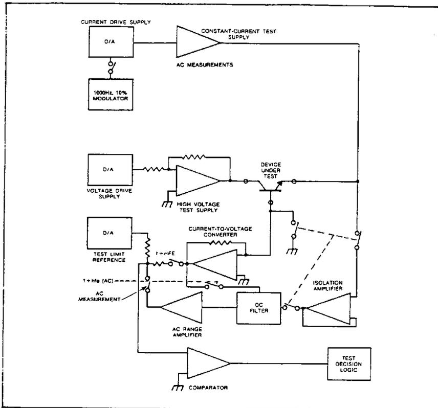
The test available are: Current Gain ( $1 + HFE$ ), and Common Base Input Impedance (HIB).
