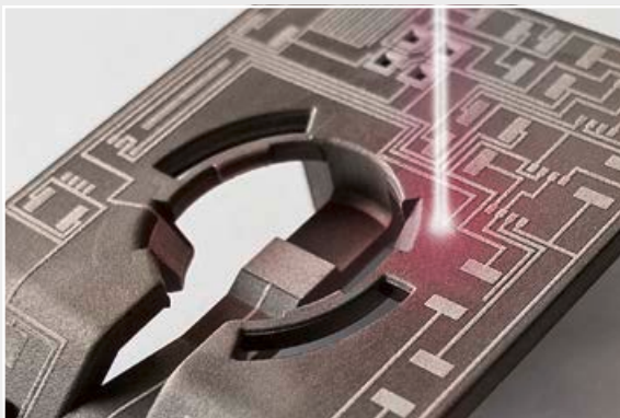
3. Structuring the circuit tracks with the LPKF ProtoLaser 3D
