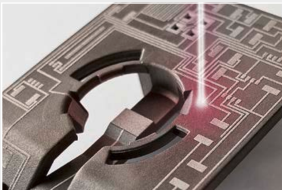
3. Structuring the circuit tracks with the LPKF Fusion3D 1200
