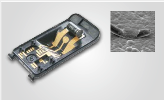
Left: Assembled component. Right: Bond on electrolessly metallized Cu/Ni/Au bond pad.
