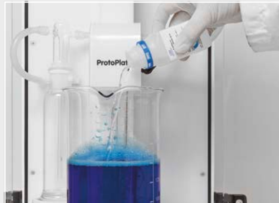
2. Pour in the activator to start the metallization bath
