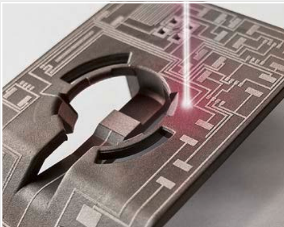
3. Structuring the circuit tracks with the LPKF ProtoLaser 3D
