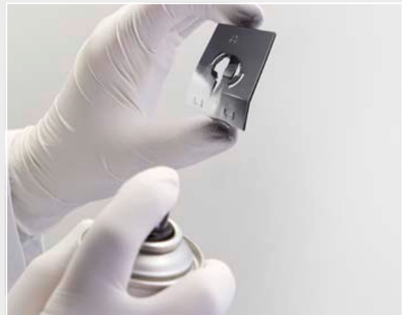
2. Painting the part with LPKF ProtoPaint LDS
