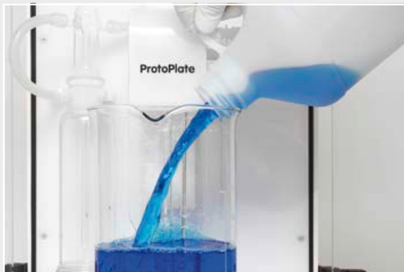
1. Pour the copper solution into the beaker
