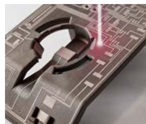
LDS prototyping stages (left to right): 3D print, coating of the base part, laser structuring, and finished 3D MID.
