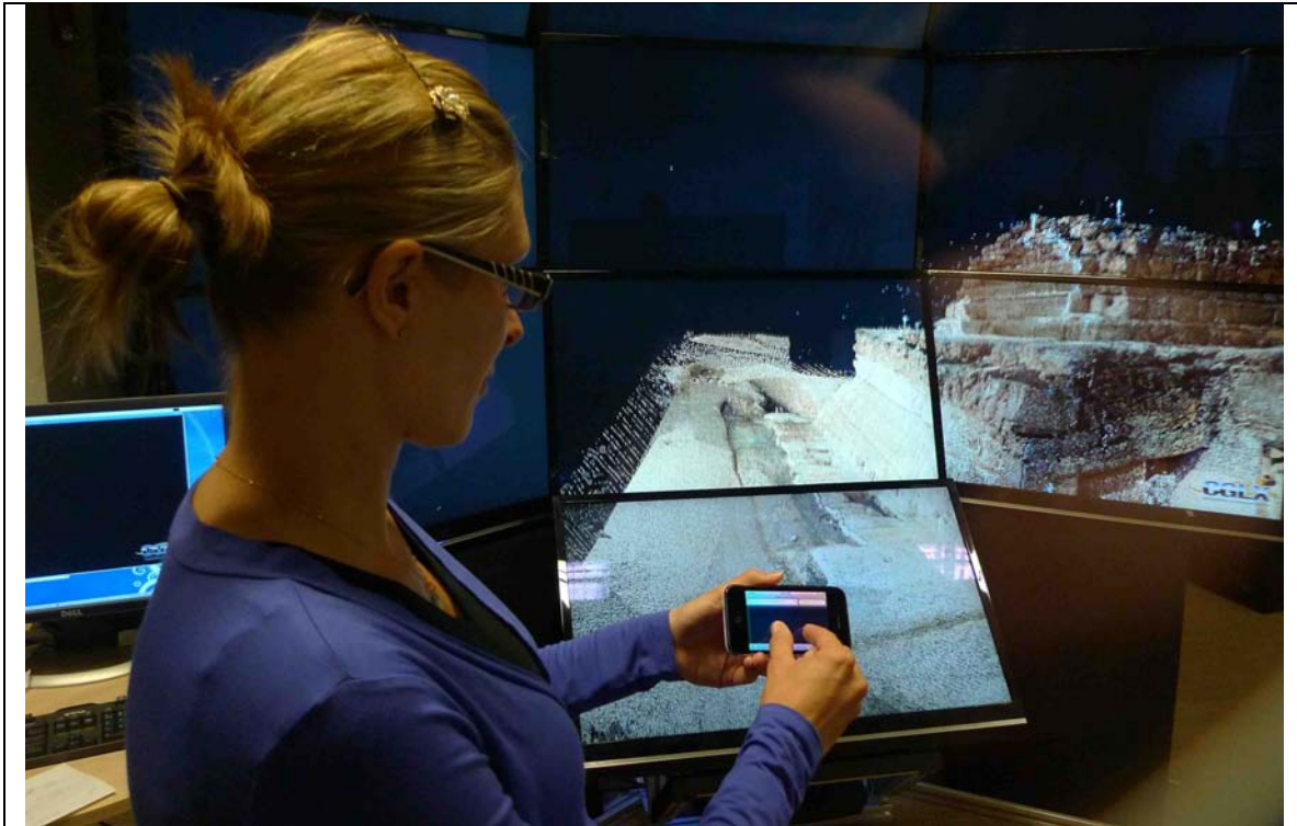
Figure 29. NexCAVE running CGLX, controlled by multi-touch iPhone application, showing LIDAR-scanned image constructed by Vid Petrovic. Photo: Tom DeFanti.
