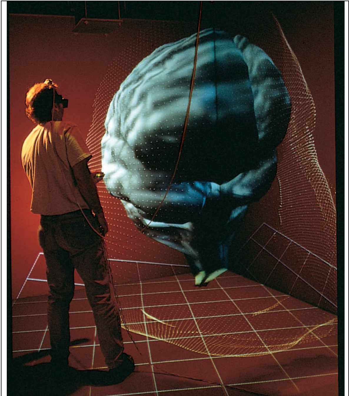
Figure 1. The “classic” CAVE is a multi-person, room-sized, high-resolution, 3D video and audio environment. Early CAVEs had less than a megapixel per wall per eye; newer ones have up to 15 times as many pixels. Photo: National Center for Supercomputing Applications at University of Illinois at Urbana-Champaign.
