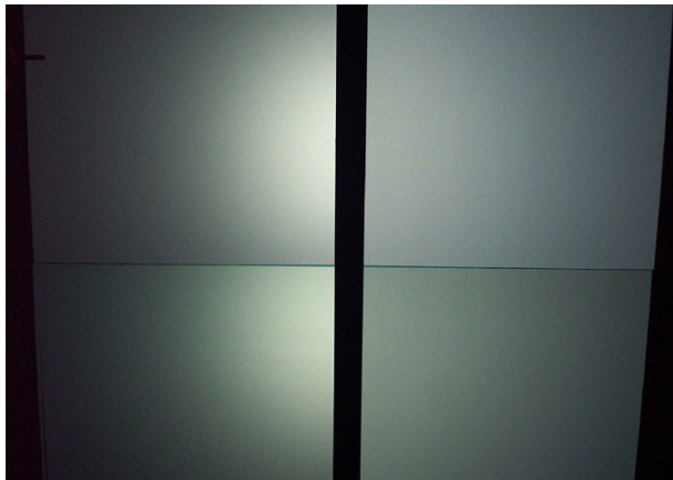
Fig. 4. Hotspotting of illumination (left) versus more even dispersion (right) on polarizing preserving screens with different coatings.
