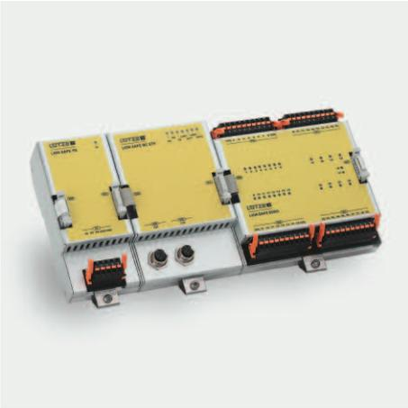
The LION SAFE Remote I/O family has been extended by a new Bus Coupler. The **LION Safe Bus Coupler Ethernet TRDP** is a Gateway between safe and non-safe I/O data from connected LION I/O Modules to Ethernet TRDP. As the system can be used for applications with a safety integrity level up to SIL2, the communication protocol can be extended with the safety frame of SDTV2.
