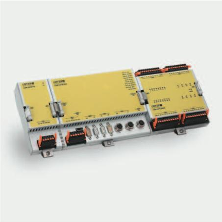
The new LION SAFE CCU is a train control unit and can be used for applications up to a safety level of SIL2. The safety-related and non-safe application software code can coexist inside of the same control unit without any cross influences.
