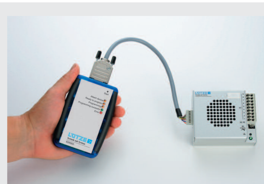
With the Programmer the Audio Signal Transducer is programmed with the Mem-file in a matter of seconds.
