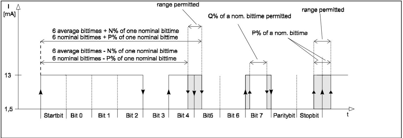
Fig. 1: Start stop distortion (example for bit 4), minimum signal element (example for bit 7) (Transmit)
