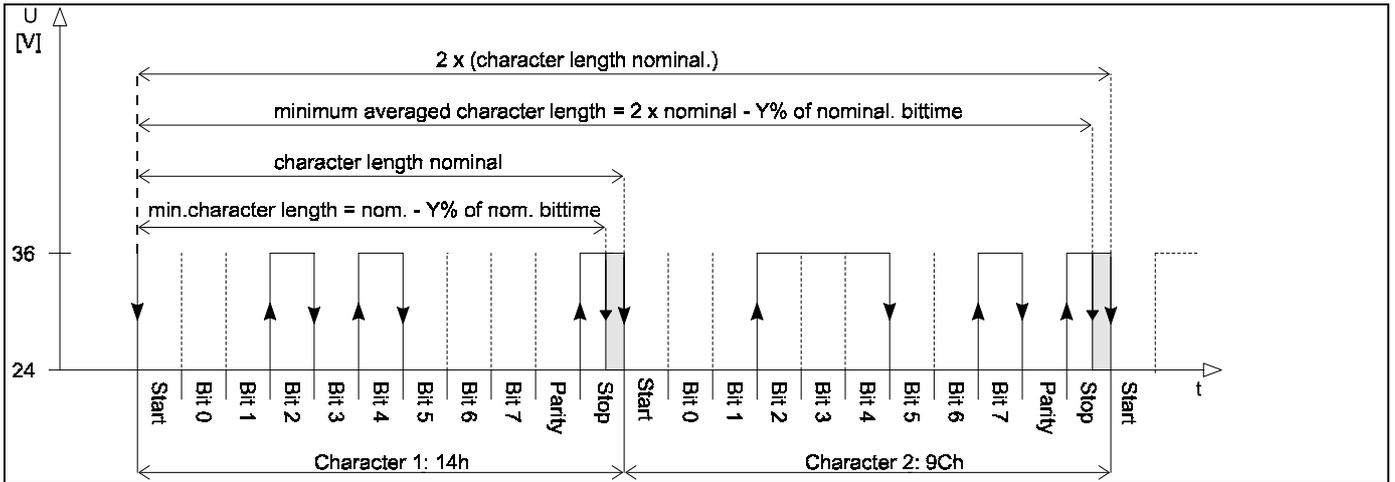
Fig. 4: Character interval requirement (Receive)
