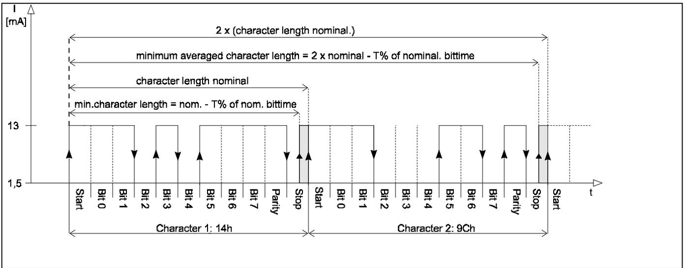
Fig. 2: Character interval requirement (Transmit)
