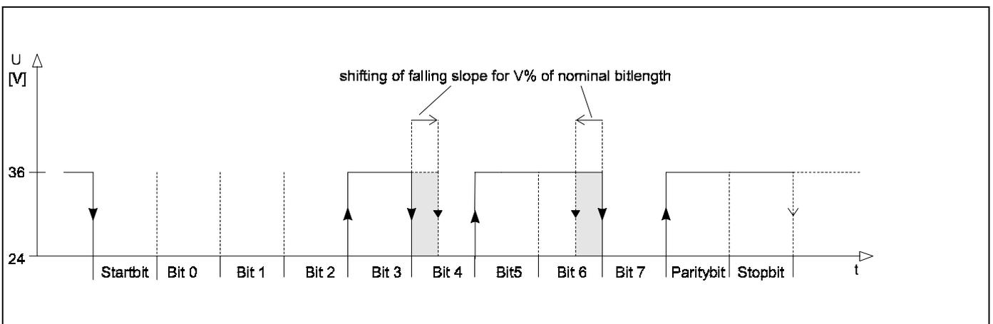
Fig. 3: Practical receive margin (example for two falling slopes)
