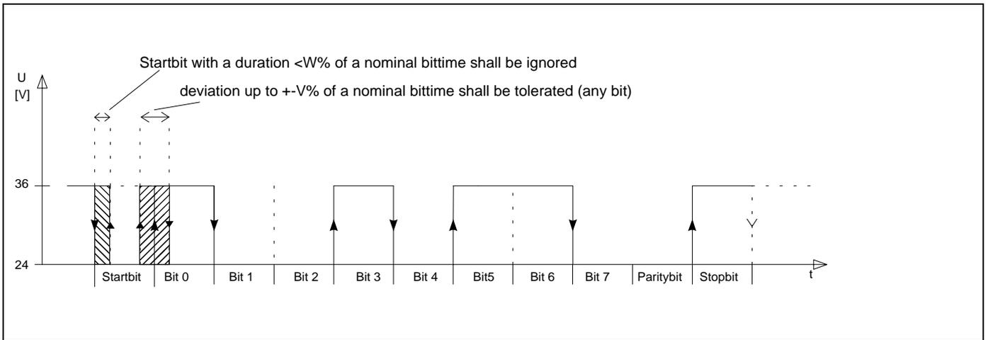
Fig. 5: Minimum duration start element (Receive)
