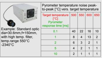
Tables show rapid improvement of signal to noise ratio for higher target temperatures and lower response time. The response time can be set by the LPM software. Please ask us for the temperature range for your application.
