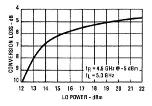
*Drive Level:* The maximum recommended drive level is +23 dBm.
