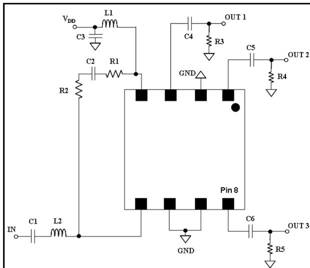
8. The exposed pad centered on the package bottom must be connected to ground for RF, DC and thermal considerations.
