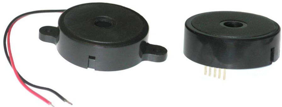
IEC 60601-1-8 compliant SBS speaker series features sound levels of 100 dB @ 10 cm in a 45 mm x 15 mm package size. Some options available with the flange mount package and all options available with pc pin terminations.
