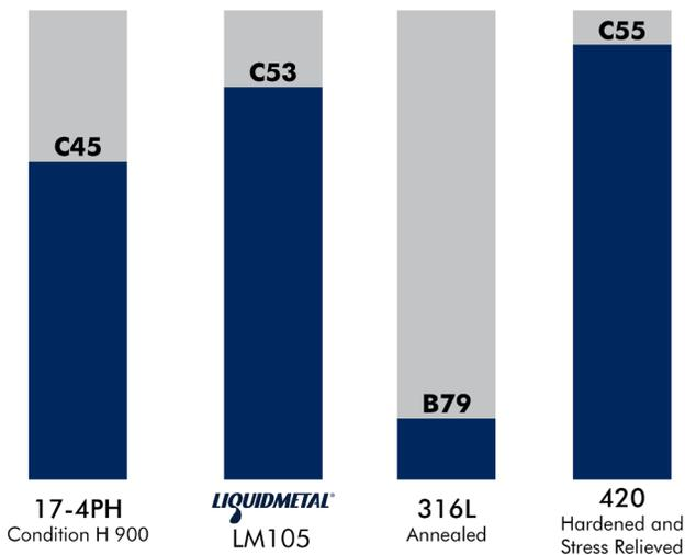
In Liquidmetal alloys, these properties are formed by the amorphous material composition. Additionally, no post mold processing is required to achieve final properties. Crystalline metals like 17-4 PH and 420 stainless steel require heat-treating to attain final properties, which can cause distortion, reduction of dimensional precision,
