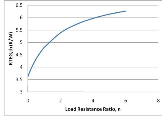
Figure 2: Plot of TEG thermal resistance as a function of electrical load resistance ratio
