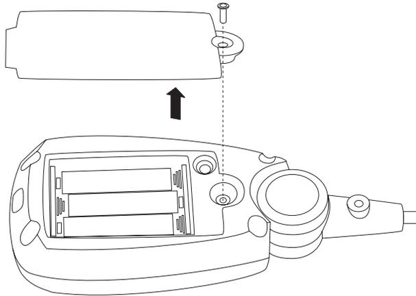
Remove the battery door to expose the three AAA batteries. Replace only with AAA batteries approved in this document. Replace the battery door and reinstall the hex screw. Be sure to use only the approved list of batteries. Any substitution will void the safety ratings of this product.
