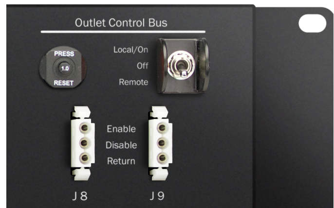
The remote switching/EPO option includes control bus connectors to match Marway's Commander UCP 3500 remote EPO panel, along with a manual override switch to force outlets either on or off.
