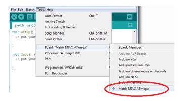
The MIAC board definition needs to be installed by unzipping the contents of the "Arduino IDE MIAC Hardware File" resource download into the "hardware" directory of the Arduino IDE installation. For example:
