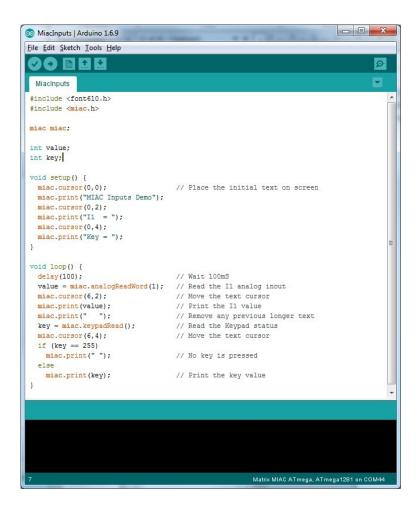
For example, the MIAC sketch "MiacInputs" demonstrates basic cursor positioning, text output to gLCD screen together with examples of how to read the keypad and the analogue inputs of the MIAC.
