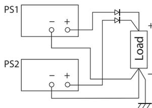
Please keep all the settings of voltage the same. Output current will be the summation of each current. Please keep OVP level of power supply maximum to prevent any damage.
