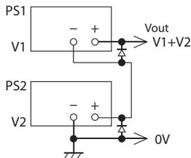
Total output voltage is to be up to 250V (-LH option models : 1kV). Therefore for models with output voltage of over 250V (or 1kV), series operation cannot be conducted. Output current is to be the smallest current of those.
