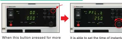
It is able to set the time of instantaneous power failure with 10 ms unit in 10 ms to 5 s by turning the rotary encoder
