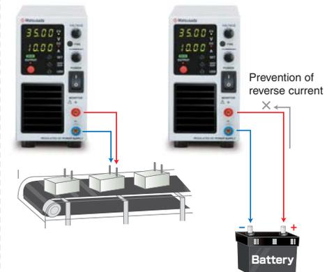
Note : It is impossible to stabilize by reverse current control. If the load is what reverse voltage becomes higher than rated voltage (induced load, regenerative motor, etc.), please protect the power supply by connecting dummy resistor, reverse current protection diode and so on.
