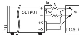
Prevent to degrade stability due to volt. drop (Vo-VL) by resistance(R) of output wiring or contact resistance. (up to max. 0.5V)
