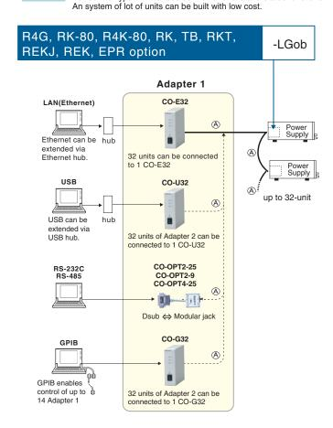
Application System when control one or several power supplies with Ethernet, USB, GPIB, RS-232C or RS-485.
