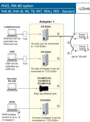
Application System when control one or several power supplies with Ethernet, USB,GPIB, RS-232C or RS-485.
