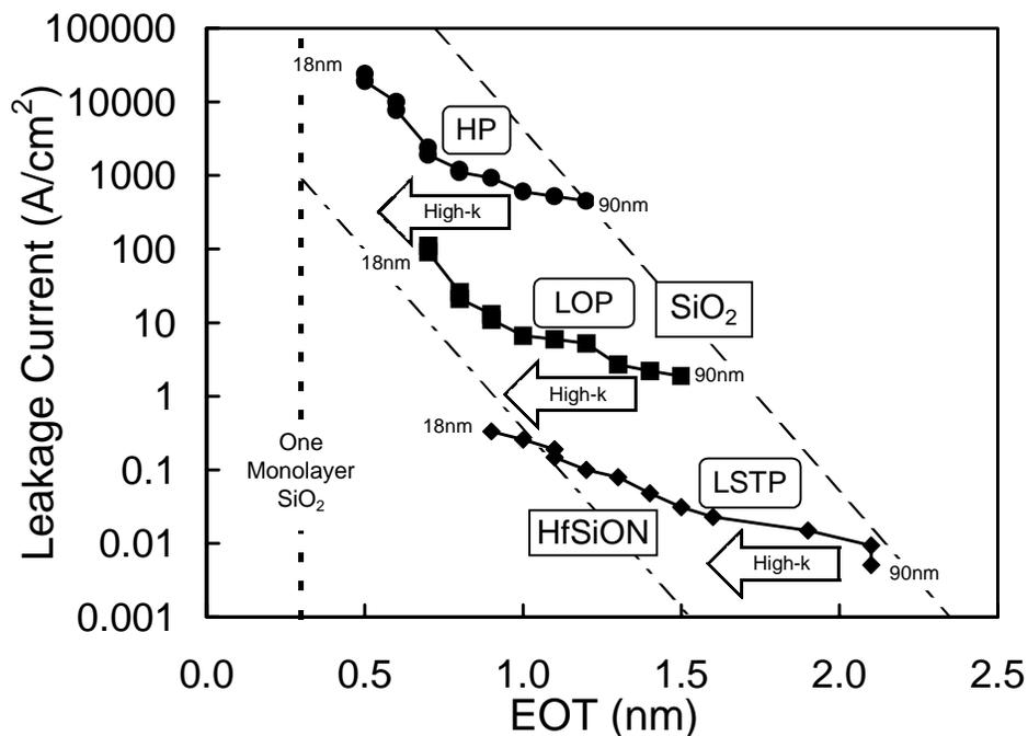
Fig. 8 Trends in the evolution of the requirements for gate dielectrics [2]. The figure shows the evolution from the 90 nm to the 18 nm node for the high performance (HP), low operating power (LOP) and low stand-by power (LSTP) families of CMOS devices. The arrows show the points where adoption of high-k becomes mandatory, according to the ITRS. The dashed lines marked SiO<sub>2</sub> and HfSiON indicate typical leakage-EOT trends expected for these materials [78].
