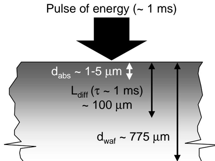
Fig.16 Critical length scales in millisecond annealing. For surface heating, the pulse of energy must be absorbed in a region ( $d_{abs}$ ) that is small compared to the thermal diffusion length ( $L_{diff}$ ). The bulk of the wafer remains cool during the energy pulse because  $L_{diff} \ll d_{waf}$ . After the pulse, the bulk acts as a heat-sink, leading to very fast cooling [50,51].
