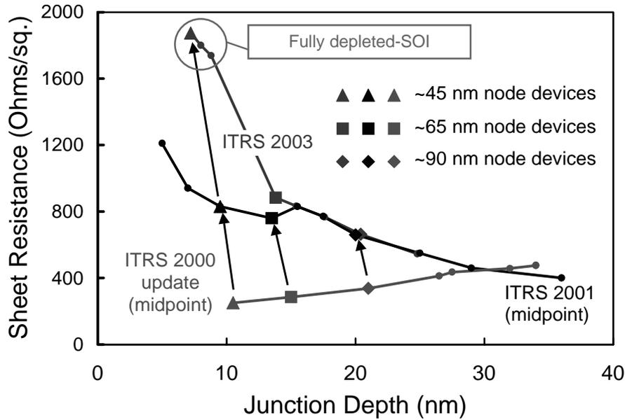
Fig. 11 Compromises in  $X_j/R_s$  requirements in recent ITRS roadmaps were necessary because of the difficulty in achieving sufficient dopant activation through conventional RTP [2,30].
