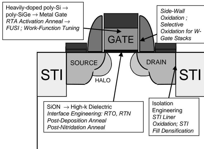
Fig. 4. Applications of RTP in gate stack and isolation engineering.
