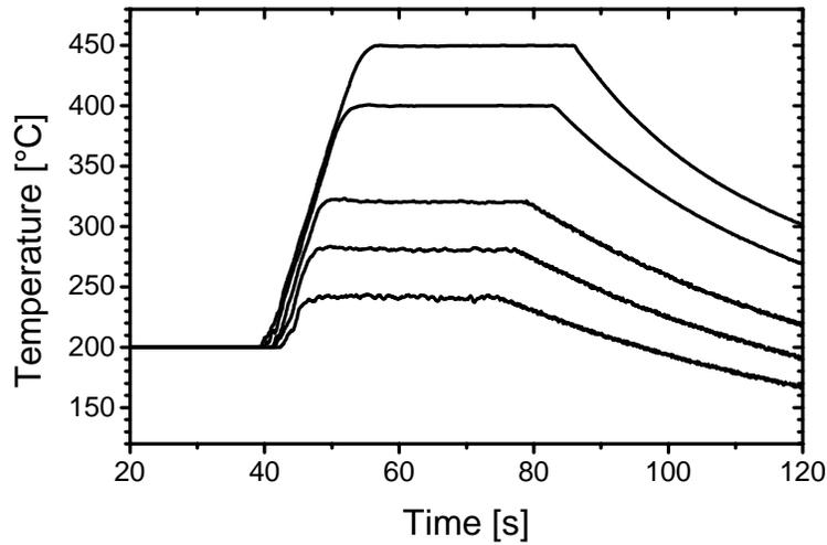
Fig. 13 Low-temperature heating cycles are becoming increasingly important for RTP processing of NiSi films (performance of Mattson Technology's Helios™ RTP system). Closed-loop control at temperatures as low as 250°C, together with relatively fast ramp-rates, will help integration of NiSi processes in advanced manufacturing.
