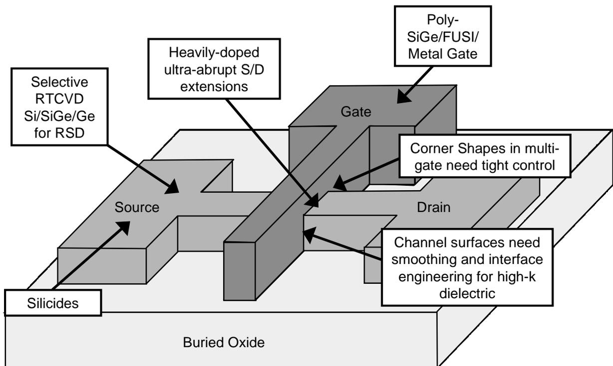
Fig. 6. RTP applications in processing of advanced multi-gate devices.
