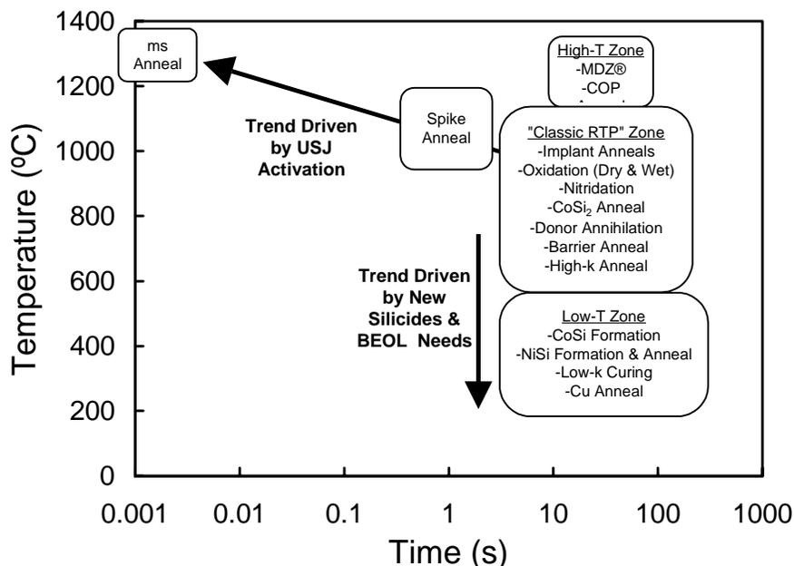
Fig. 7. The temperature-time domain of RTP continues to evolve. Recent trends include “hotter and faster” processes that enable the creation of advanced ultra-shallow junctions and low-temperature processing that is needed for NiSi formation and annealing.
