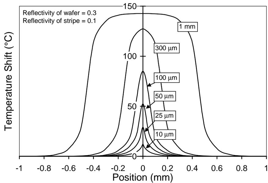
Fig. 17. Predictions of the pattern effect in pulsed heating [115]. The curves show the temperature non-uniformity expected to arise when a region that contains a stripe of absorbing material is exposed to a 1 ms duration pulse that produces a 500°C temperature rise on plain silicon. The numbers in boxes are the stripe widths. The absorbing region heats to a significantly higher temperature than the neighbouring silicon, producing a large pattern effect.
