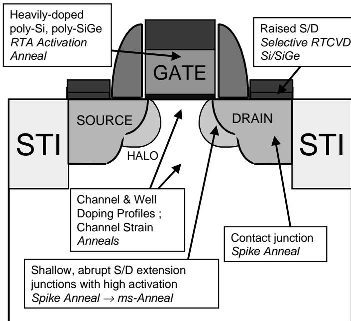
Fig. 3. The role of RTP in advanced doping and strain engineering.
