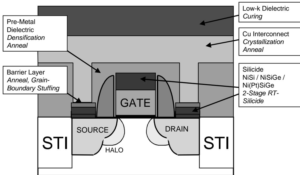
Fig. 5 RTP applications in contact and interconnect engineering.
