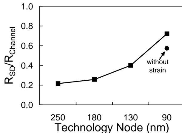
Fig. 9. The ratio of the source/drain resistance to the resistance of the transistor channel has been rising rapidly through successive technology generations [8]. Innovations such as strain, that help increase channel mobility, will exacerbate the trend. Ultimately, the parasitic resistance will limit device performance. New approaches for dopant activation and contact formation are essential to overcome this challenge.
