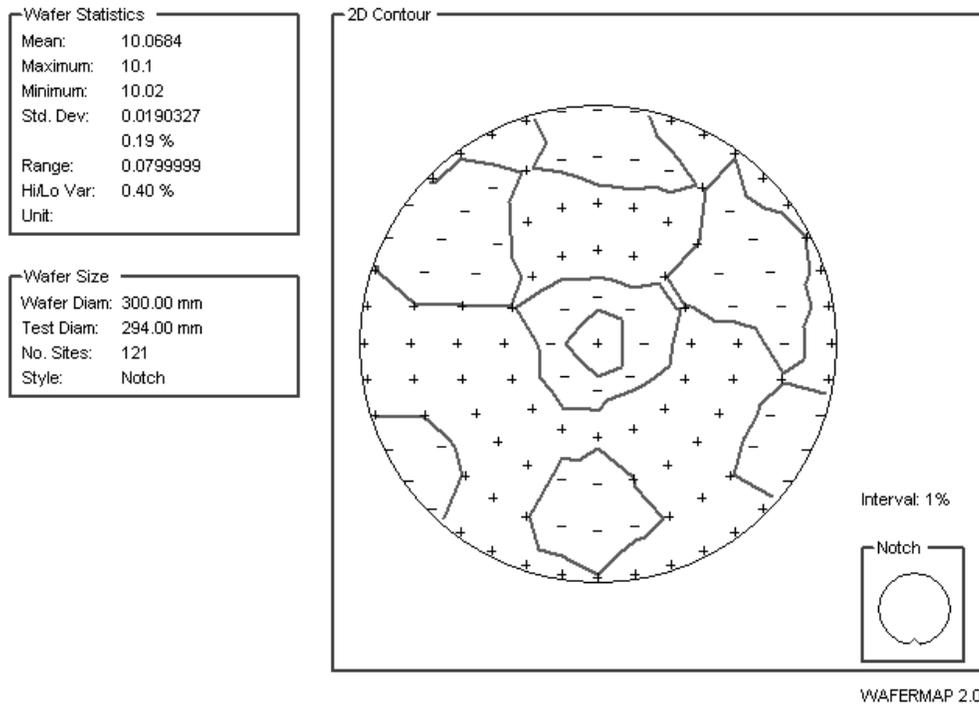
Fig. 14 Modern RTP systems can provide extraordinary within-wafer uniformity. This process result is from Mattson Technology's Helios™ RTP system. The temperature range from the RTO process of 60 s at 1100°C corresponds to a total temperature range of only 1.05°C across the 300 mm wafer.
