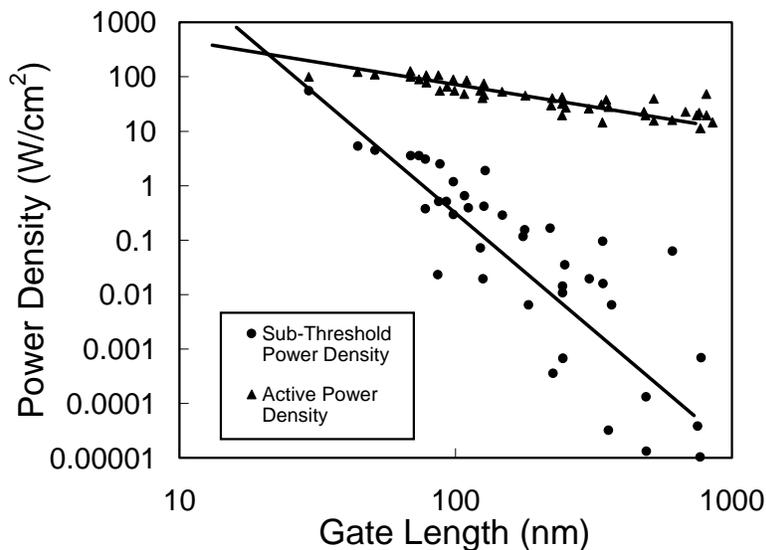
Fig. 2. MOS device power trends [4]. As devices have scaled below the 90 nm node, CMOS ceases to be a “power-friendly” technology, mainly because of the very rapid rise in the “off-state” leakage currents. Continued progress will require increasingly sophisticated approaches, including the use of new materials, device architectures and circuit designs optimized for power-management.
