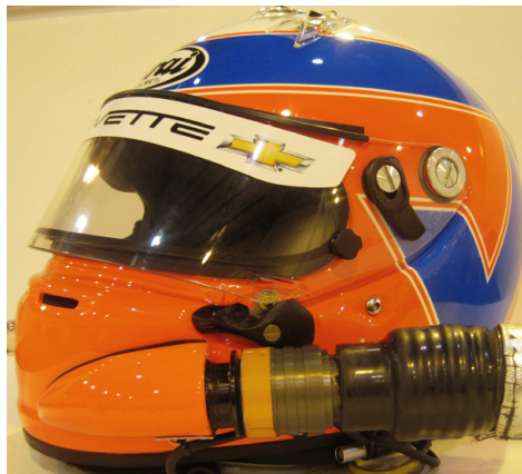
The actual driver's helmet showing the connector parts designed using NX software.
