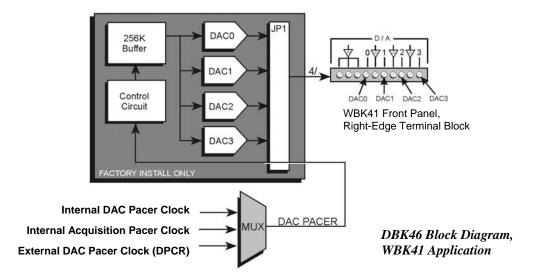
The DBK46 has a 256K sample buffer that can be used for one to four DACs. If only one DAC is enabled for waveform output, then the entire 256K sample memory can be used to store a waveform for that DAC. If two DACs are enabled for waveform output, then 128K of sample memory is available for each of the two DACs. Use of all four DACs drops the available memory down to 64K per DAC.
