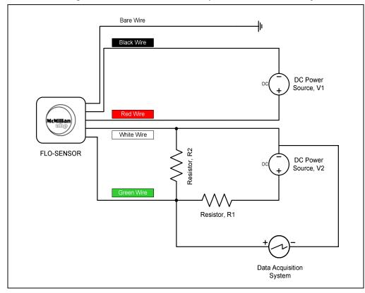
Wiring Schematic For Isolated Pulse Output. "A" or "E" Suffixes Only
