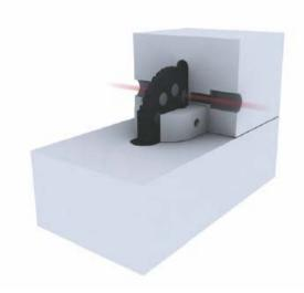
McMillan's patented technology measures flow using a miniature turbine wheel approximately 0.8 inches (20 mm) in diameter. The micro-turbine wheel is supported on a very small sapphire shaft that is held in position by two sapphire bearings. The micro-turbine assembly is so light that it virtually floats in the liquid. This relieves force on the bearings and eliminates wear. Consequently no particles are generated.
