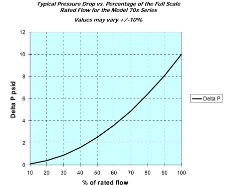
For example: You have a sensor with a 50-500 ml/min flow range (Range 5) and want to know the pressure drop (or minimum differential pressure required) at 300 ml/min. According to the calibration certificate, the pressure drop at 100% of flow is approx 10 psi. Using the formula above:
