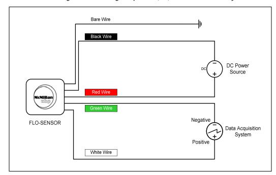
Wiring Schematic Voltage Outputs. "B", "D, "J" or "K" Suffixes Only
