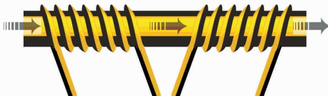
**Figure 4: Sensing Coil on McMillan Thermal Sensors**
