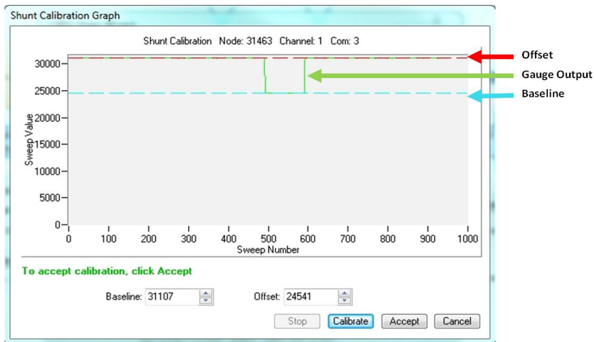
Figure 69 - Strain Gauge Calibration
