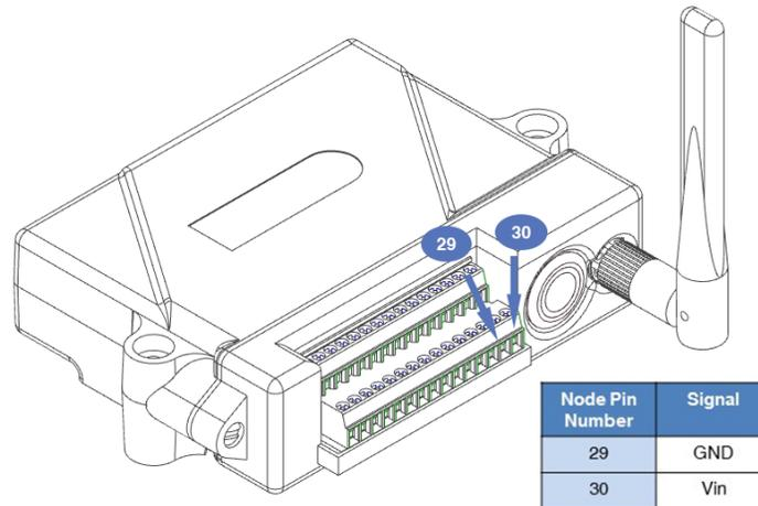
Figure 50 - External Power Connection
