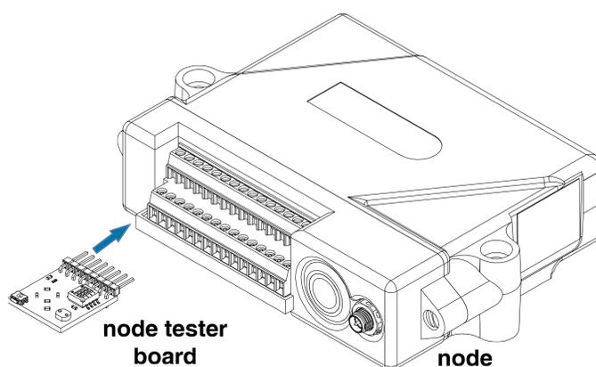
Figure 51 - Node Tester Board Installation
