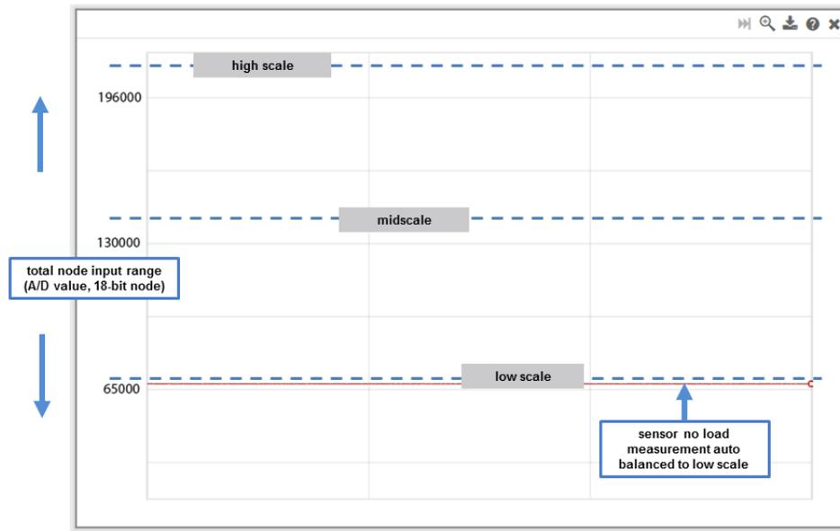
Figure 45 - Offset Scale Setting
