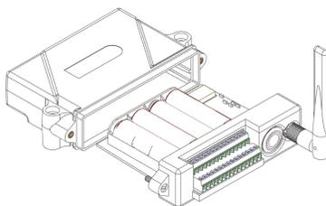
Figure 58 - Replace Batteries
