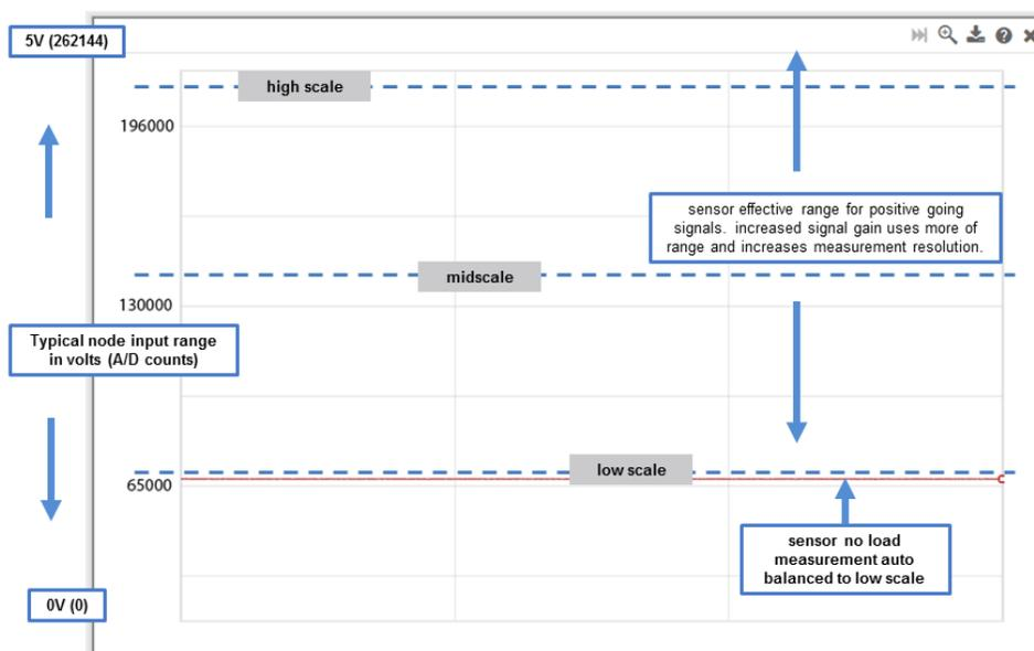
Figure 49 - Differential Input Resolution and Offset (18-bit Node)
