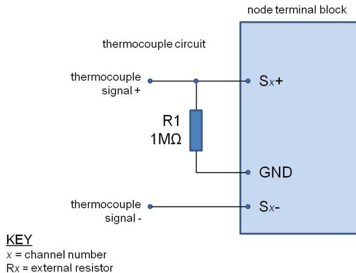
**Figure 35 - Connecting a Thermocouple**
