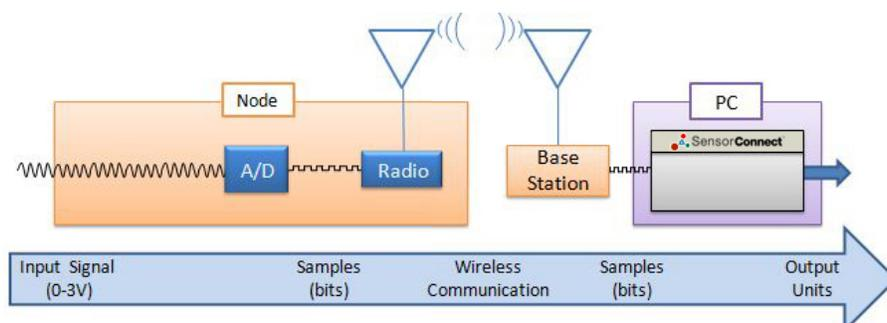
**Figure 33 - Single Ended Signal Processing**
