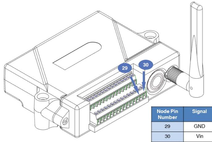
Figure 50 - External Power Connection
