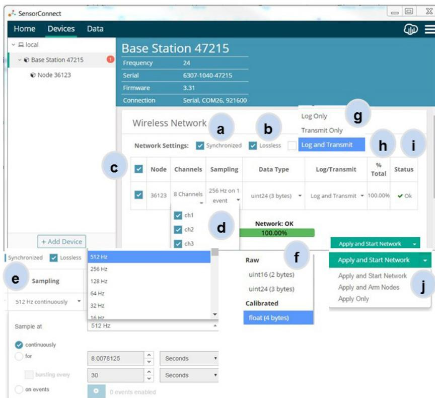
Figure 15 - Network and Node Configuration Menu
