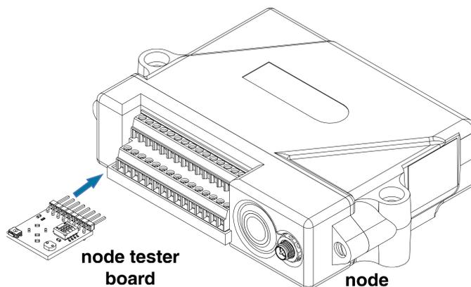
Figure 51 - Node Tester Board Installation
