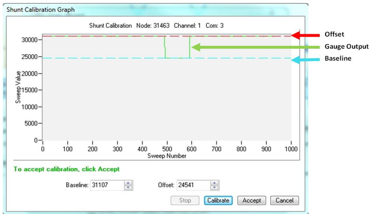
Figure 50 - Strain Gauge Calibration
