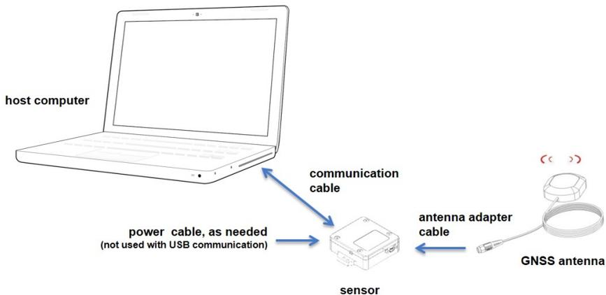
Figure 4 - System Connections
