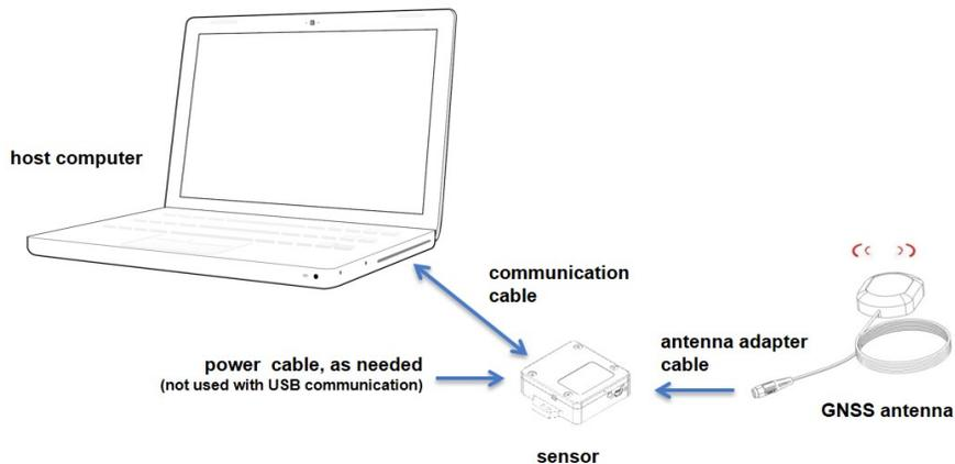
Figure 4 - System Connections
