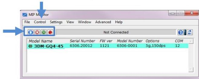
Figure 10 - Main Window Controls
