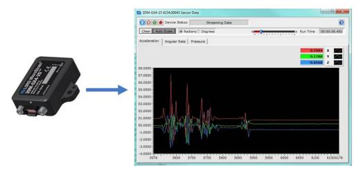
Figure 3 - Acquiring Sensor Data with MIP<sup>™</sup> Monitor
