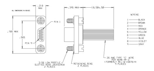
Figure 37 - Connecter interface cable (sold separately, PN: 6224-0100)
