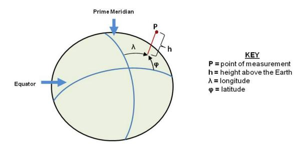
Figure 18 - World Geodetic System (WGS84) Reference Ellipsoid
