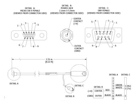
Figure 35 - Communications and power cable (RS232 Kits, PN: 4005-0037)
