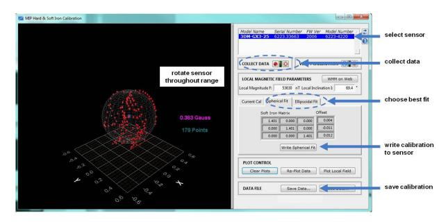
Figure 24 - Collect Calibration Data
