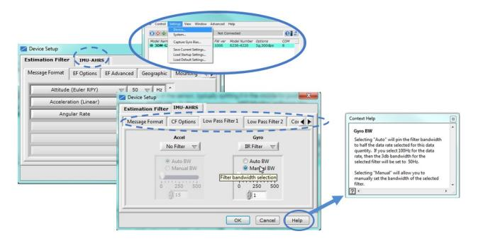
Figure 16 - IMU Settings
