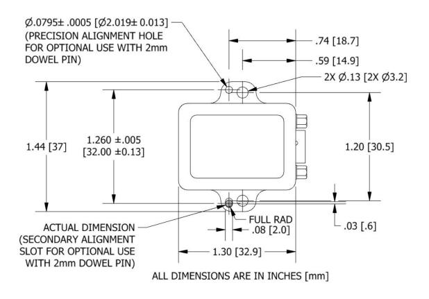
Figure 28 - Mounting the Sensor
