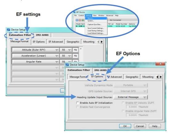
Figure 27 - Heading Source Setting
