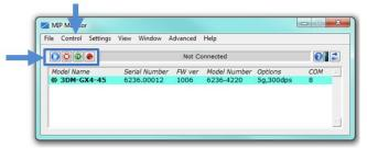
**Figure 11 - Main Window Controls**
