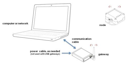
Figure 4 - System Connections
