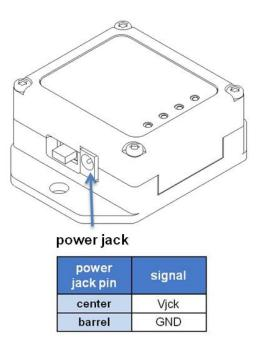
Figure 28 - External Power Connections
