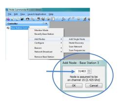
Figure 6 - Adding a Node by Address
