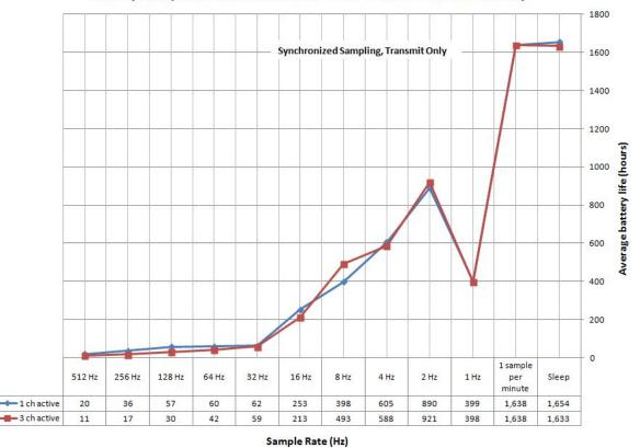
Battery life aproximation for G-Link<sup>®</sup> -LXRS<sup>®</sup> 220mAH internal battery
