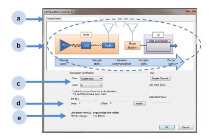
Figure 9 - Channel Setup
