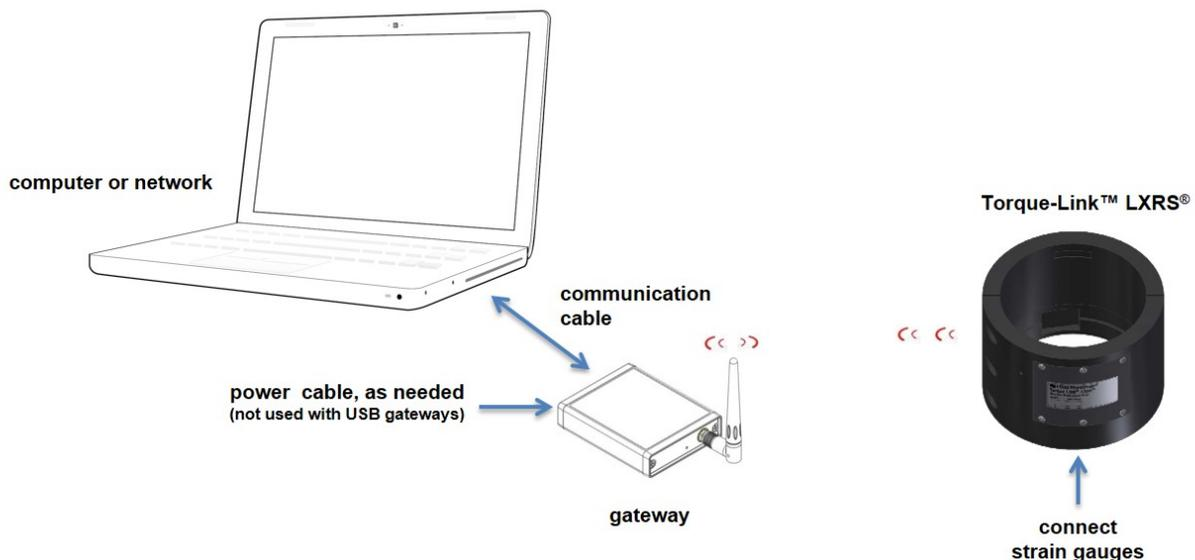
Figure 6 - System Connections
