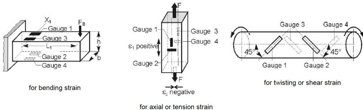
**Figure 27 - Example Gauge Placement**
