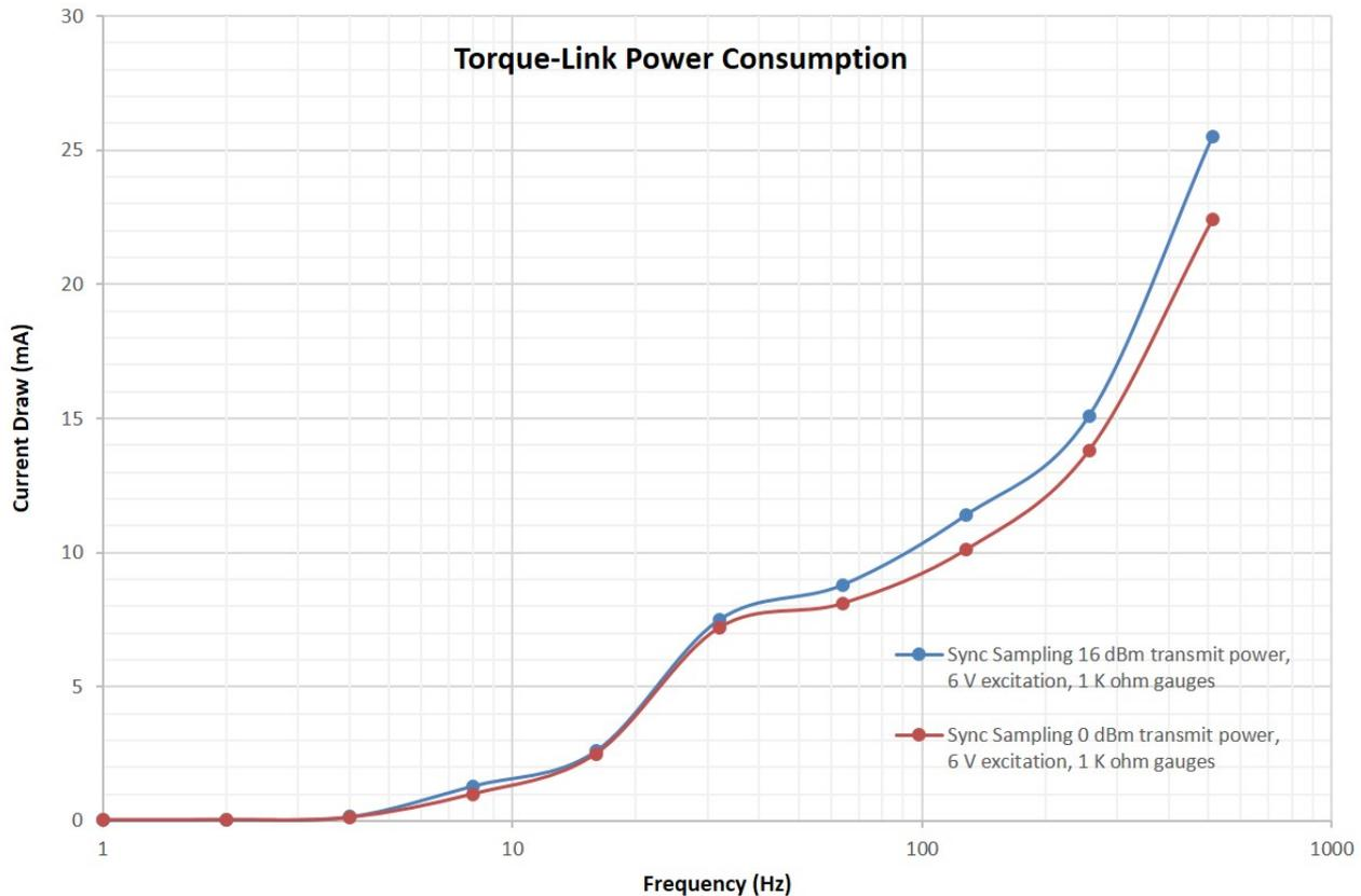
Figure 54 - Example Torque-Link™-LXRS® Power Profile
