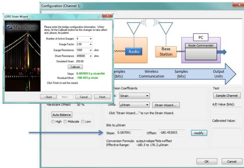
**Figure 35 - Completed Strain Wizard**
