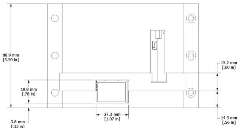
Figure 29 - Strain Gauge Placement
