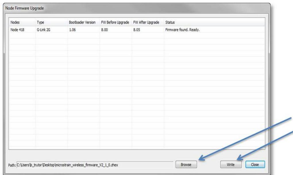
**Figure 50 - Upgrade Firmware Window**
