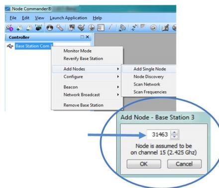
Figure 8 - Adding a Node by Address
