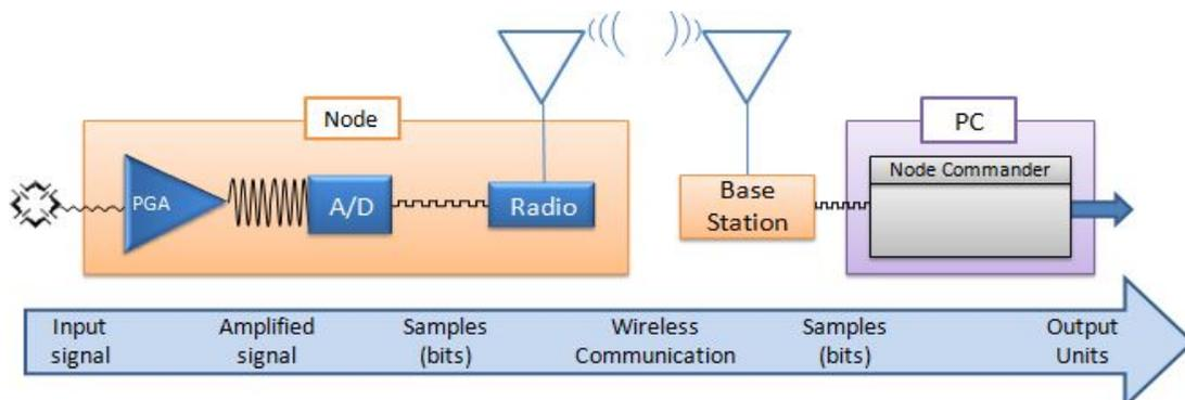
Figure 24 - Differential Channel Signal Processing
