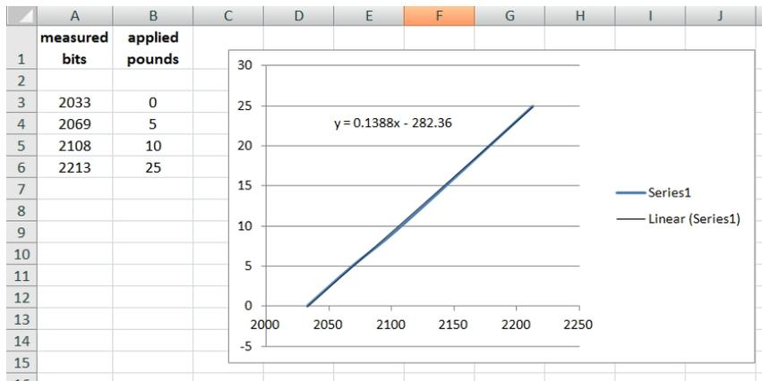
Figure 44 - Slope and Offset Values
