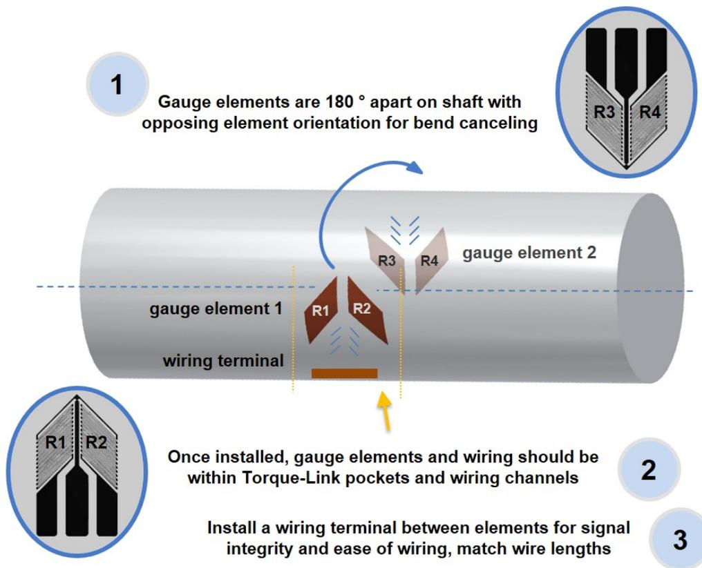
Figure 28 - Placement for Full Bridge Torque Measurements
