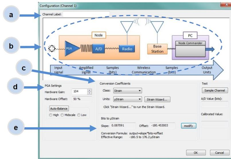
Figure 11 - Channel Setup
